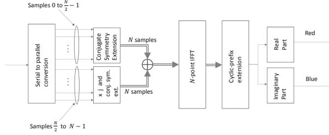
Figure 1: Transmit-side with improved IFFT processing.
