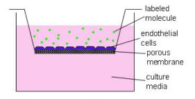
Figure 1: Experimental setup for endothelial permeability measurements.
