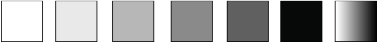
Fig. 3: Laser-printed filters for gels. The first six on the left will create control gels with a uniform stiffness. The last filter on the right is for creating the experimental gel with a stiffness gradient.
