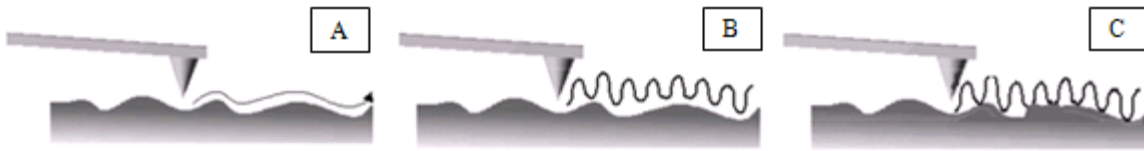
Figure 5. (a) Contact mode; (b) Non-contact mode; and (c) Tapping mode. [6]
